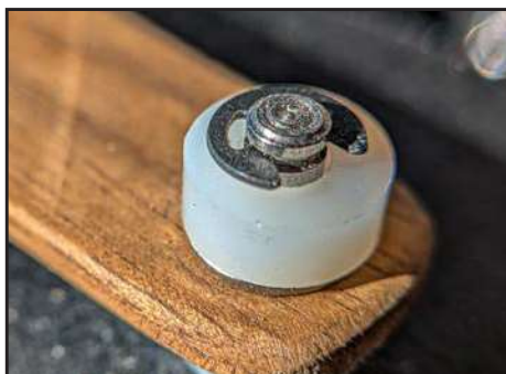
2. An e-clip at work, retaining a rolling wheel on a shaft.
