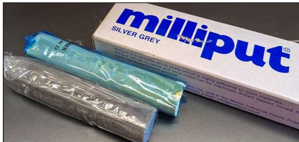
3. To use Milliput, cut two equal amounts and knead them together until they are a smooth, single color. This epoxy putty cures slowly, giving you several hours of working time.
