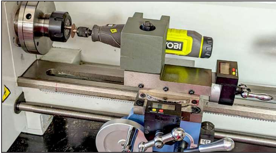
5. The rotary tool is held firmly on the compound slide of the lathe. This arrangement allows the rotary tool to be precisely positioned.
