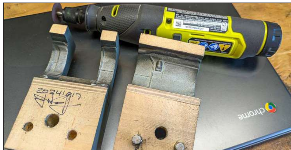
4. The rotary tool's shape has been perfectly impressed into the Milliput.
