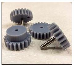
These internal spur gears were filament printed.
