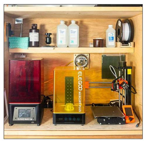
This is my 3D-printing cabinet, with the doors removed. Under the red cover is the resin 3D printer and under the yellow is the alcohol-wash station for the resin prints. The filament printer sits at the right. The cabinet keeps shop dust out and also provides a sort of climate that I can control. I can heat it and keep the drafts away from the printing process. Resins, filaments, alcohol, and wipes sit on the shelf.
