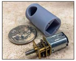
I needed a way to mount this small gear motor. 3D printing came to the rescue with the gray housing.
