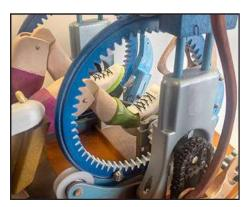
These are 3D-printed resin spur gears that I designed using FreeCAD. It is my experience that these gears are very precise, strong, and reliable.
