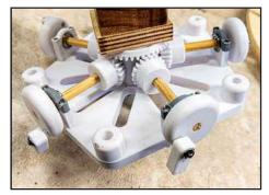
This is the gear head for a carousel. There are both filament- and resin-printed components in this complex piece. The carousel has operated flawlessly under power for hundreds of hours.
