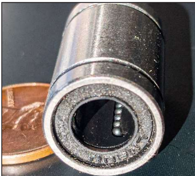
One of my automata operated a Nordic Track (ski machine)-sort of mechanism. Linear-motion bearings like this one were used. In this image, you can see the small bearings that recirculate as the bearing moves along the shaft.
