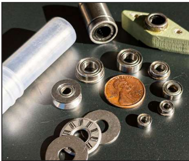
Shown here is a sleeve of 10 ball bearings, a linear ball bearing, a one-way ball bearing, a thrust bearing, a grooved bearing, and six bearings that I commonly use.
