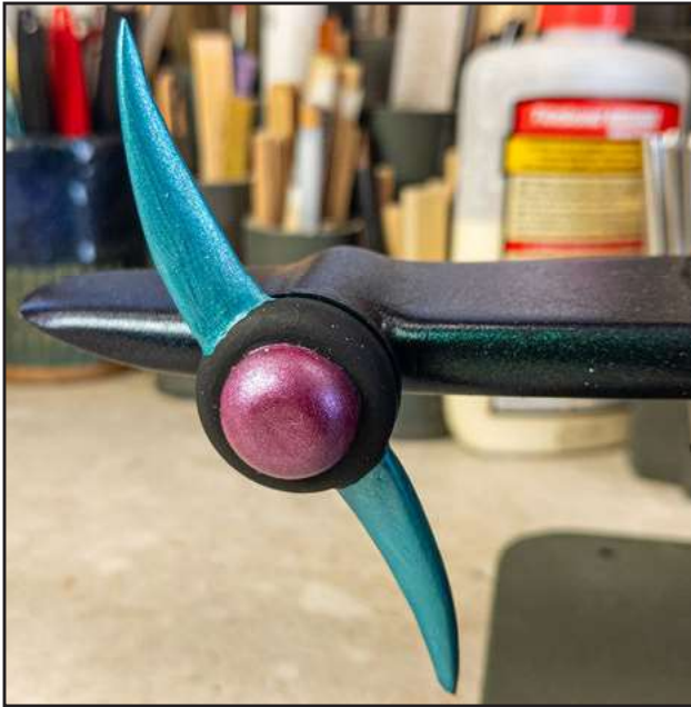
8. This propeller is magnetically held in place via an infirm connection.
