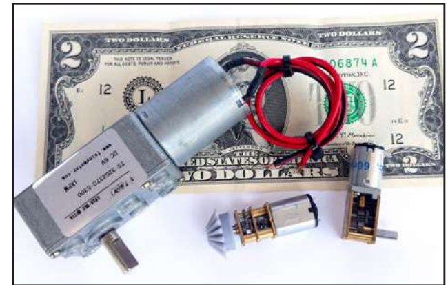
2. DC gear motors can also be used to power automata. My favorite is the large one. Note that gear motors can have shafts in different orientations.
