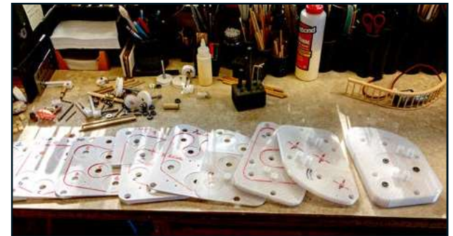
3. One of the great things about 3D printing is the ability to easily modify parts. This image shows nine iterations as I sought the perfect drive frame.
