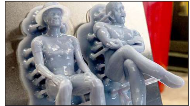
3. Two freshly printed figures. The next steps include an alcohol bath to remove uncured resin, then the removal of the supports that cradle the figure during the printing process. They are easily removed.
